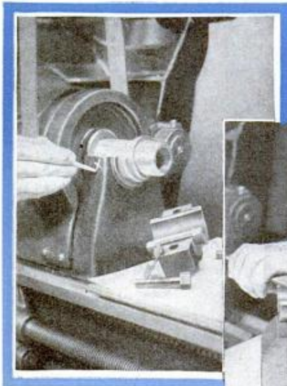
The front bearing cap and the headstock are marked with chalk so the cap can be replaced without difficulty in the proper position
