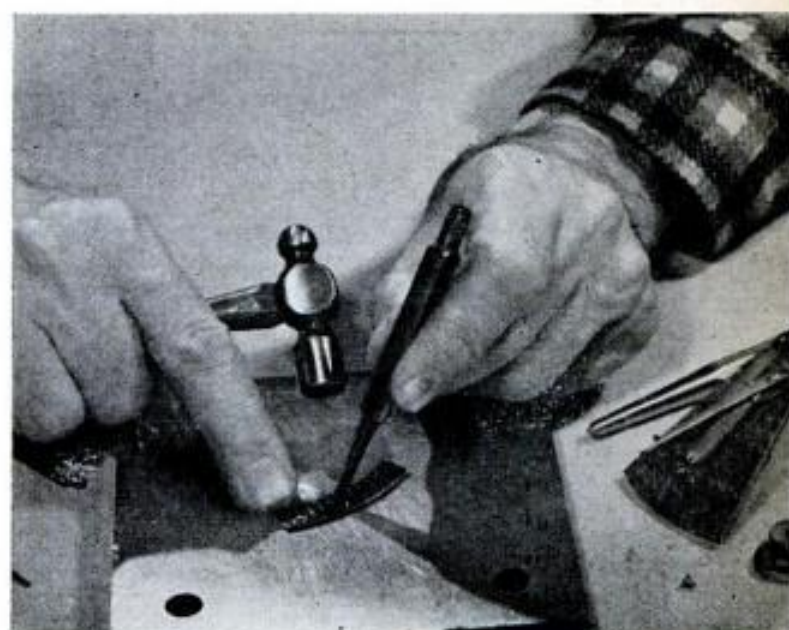
PERMANENTLY SCRIBE the calibration marks on the scale plate by using a punch and a fine-edged chisel
