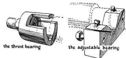
The thrust bearing of a traveling microscope
