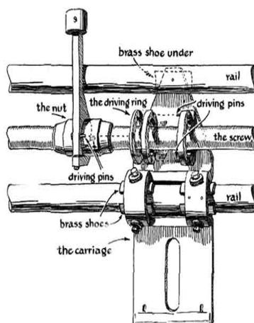
The carriage assembly of a traveling microscope
