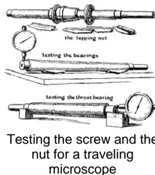
achieved. The outside of the nut was tapered so that steel rings could be slipped on to hold the nut segments together. Being rigid, they tended to produce a screw of uniform diameter.
